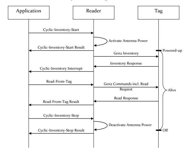
In this sequence the tag is not powered twice and is immediately operated when it is detected. This means that the tag gets the read command in exactly the same circumstances (frequency, distance, etc.) like it was detected.
